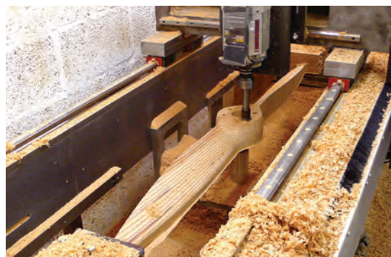
Right: Propellers are machined to exact parameters from CAD models with the aid of a purpose designed CNC machine and then hand finished.
